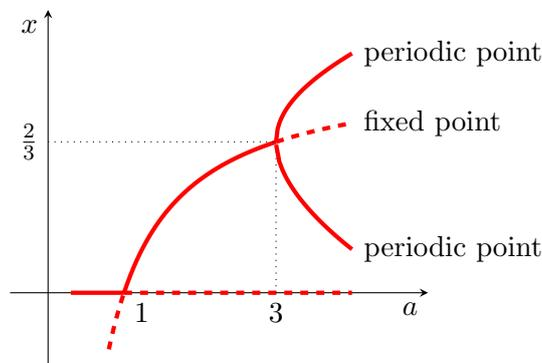
Figure 4.12: A snapshot of the bifurcation diagram from Example 4.9, given by the logistic map with  $a = 3$ .
