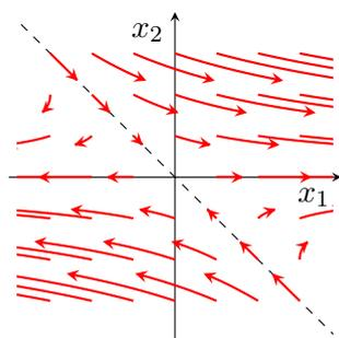
Figure 8.3: The phase portrait of the solution from Example 8.24. The first eigenvector spans the  $x_1$ -axis, and the second eigenvector spans the dashed line given by  $x_2 = -x_1$ .
