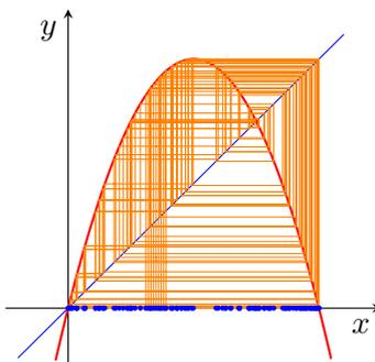
Figure 6.4: A demonstration of the topological mixing property of the logistic map for  $a = 4$ . Here, the open set is  $(0.3, 0.4)$ , and we plot 20 iterations of eight paths. We color points in the orbit on the  $x$ -axis in blue.
